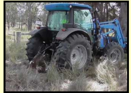
↑ Use a machine with a ripper or a bucket to destroy the burrows
